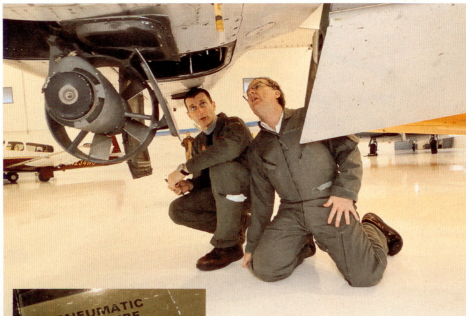
Preflight demands a check of the ram air turbine (left), pneumatic pressure (far left), and a look inside the variety of other access panels.
