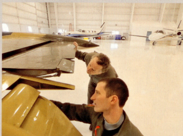
The author and Greg Morris review the aircraft flight envelope during ground school (left). The L-39's Fowler flaps are clearly visible during the preflight inside Gauntlet Warbird's hangar at Aurora Municipal Airport (right).
