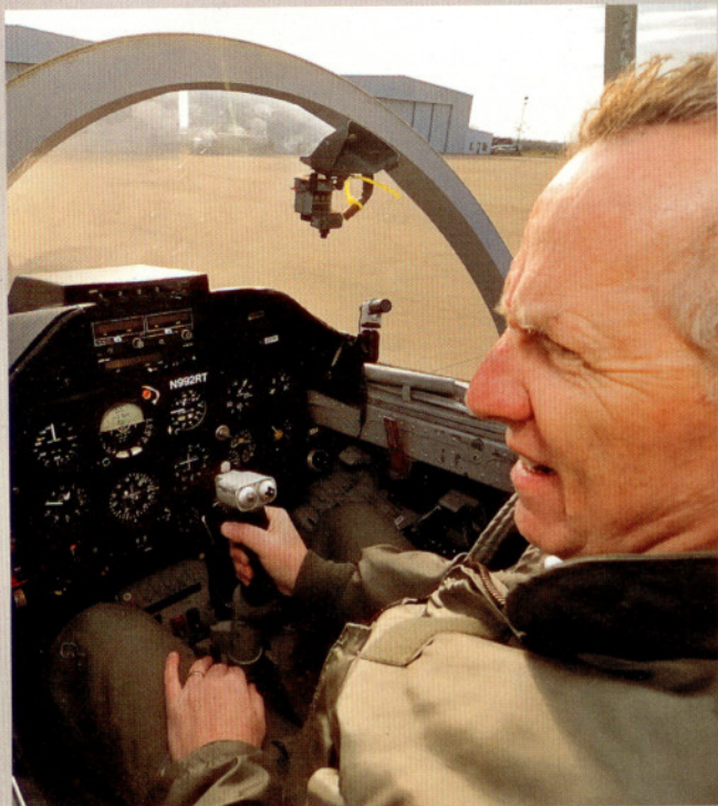
The panel on the L-39 is a conglomeration of normal gauges, except some are labeled in English, others still in Cyrillic.
